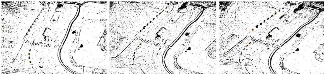
Figure 2. Binarized and unsharp masking added frames of the video.
