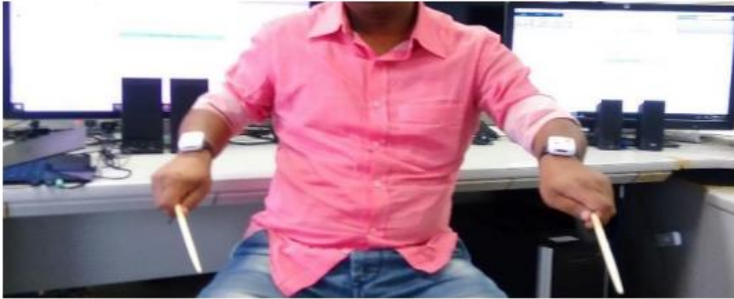
Fig. 14. Playing virtual drum by using MEMS 3D accelerometer sensors
