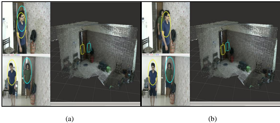
Figure 1. Results of the proposed method. The two images on the left of (a) and (b) are from the dual-view camera system, which shows humans detected with a particular color bubble (label).
