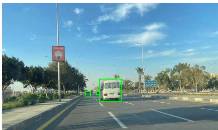
Figure 7. the application of the proposed method was successful in detecting objects in the scene while prioritizing objects in the foreground for sooner detection compared to further objects
