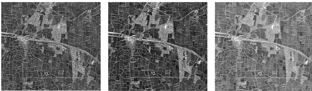
Fig1:(a) DMSAR processed image (b) Median Filtered (c) Median + Lee Filtered
