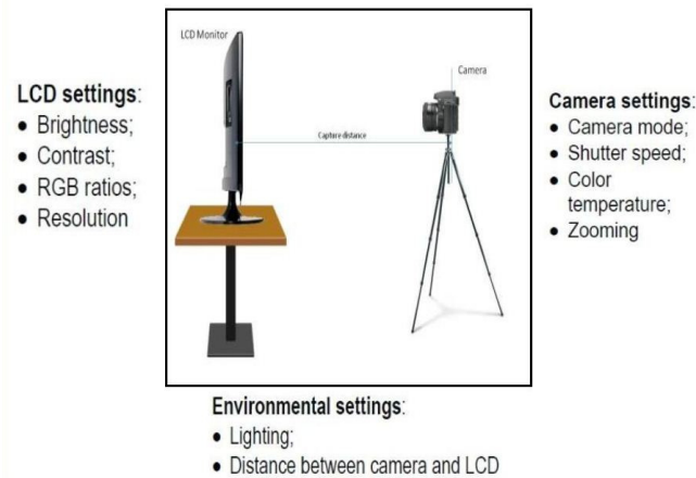
Figure 4. Some controllable settings for reproduction process on a LCD screen
