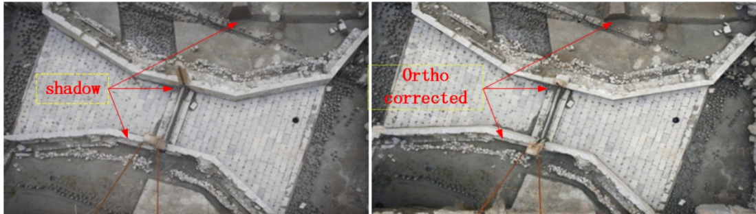
Figure 9. Airborne remote sensing image of a sluice on the Grand Canal before and after orthographic projection
