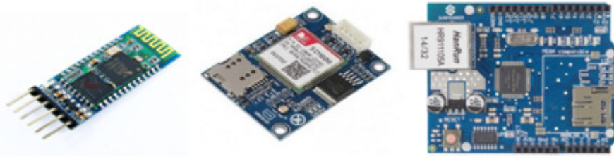
Figure 10 Bluetooth HC-5 device Figure 11 SIM808 Module Figure 12 Ethernet shield
